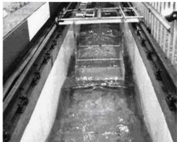
Figure 1 - General view of the experimental set-up: trolley with inclined plate in wave channel
