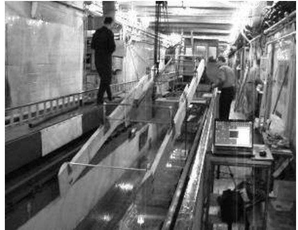
Figure 12 - Catamaran with jet-wave propeller is being lowered to the water surface in the channel
